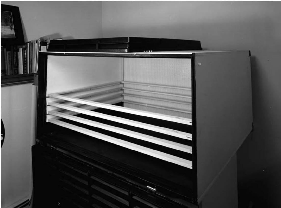
The HEPA filtered Dryer
